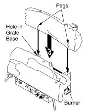
Figure 26 - Installing Rear Log (#3) (CCL3930PR/NR Shown)
